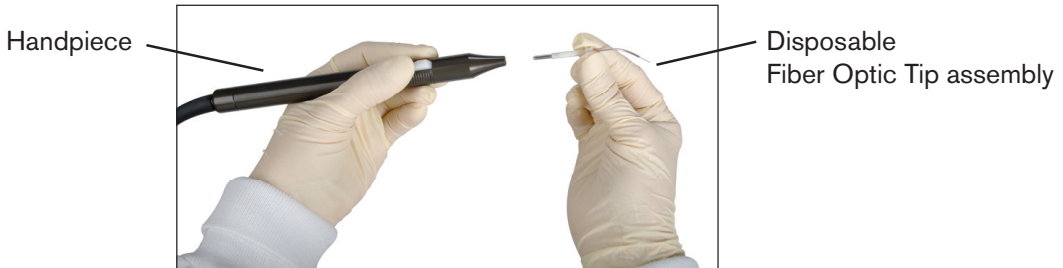
Installing the Fiber Optic Tip
