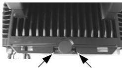
2. Remove the pole cover on rear edge of the base top cover of FT system by first removing the 2 arrowed screws in the left picture and then pushing the wedge shaped pole cover up.
