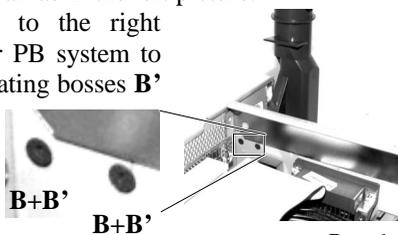
8. Please note the importance of keeping the leftward pressure on bottom end of pole display during the process of turning the pole upright and inserting the locating bosses **B'** or even when you want to release the locating bosses **B'** away from I/O plate **B** and turn the upper end of pole display to left to remove the locking lugs **A'** from bottom chassis **A**. Ignorance of this point may damage or even break off the locking lugs **A'** due to improper torque applied.
