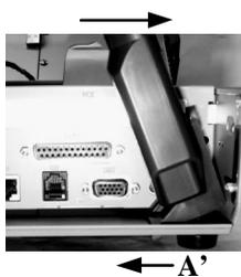
6. Please always keep a gentle pressure at the bottom end of pole base (bottom locking lugs **A'**) to the left (away from the sidewall of system chassis) when moving the upper part of pole toward sidewall as in the left picture.
