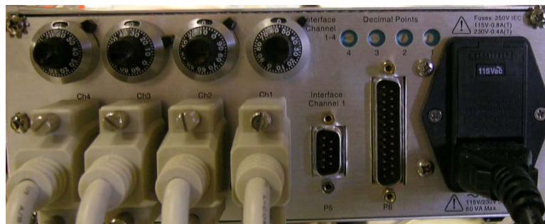
Fig.4. MKS 247D four-channel readout box, (Top) front panel, (Bottom) rear panel.
