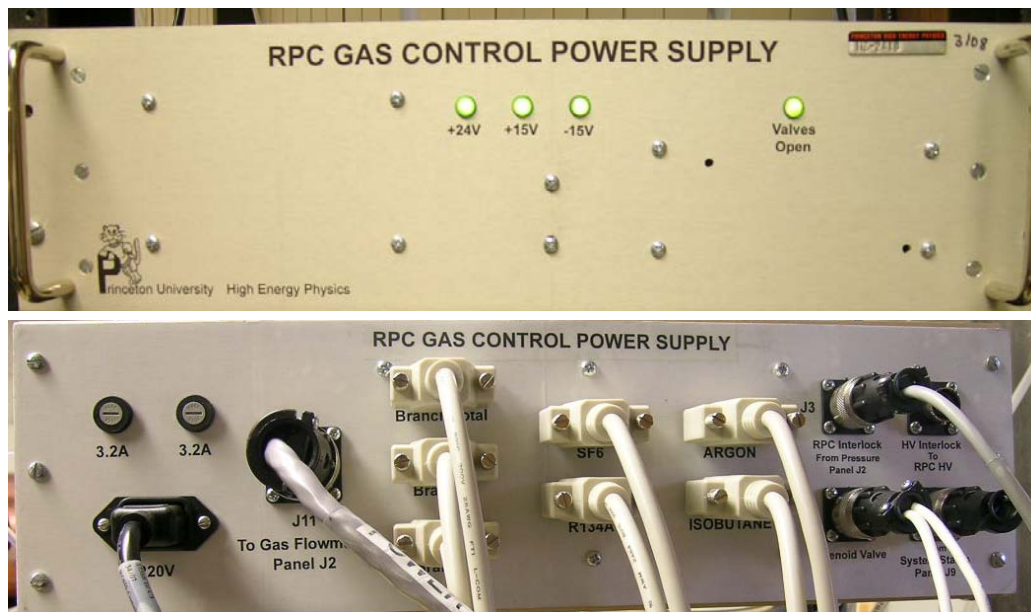
Fig. 14. Front and rear view of the power supply crate.
