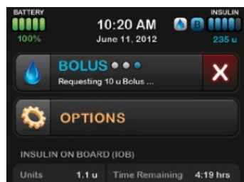
The t:slim confirms each bolus (above) and provides ten seconds to cancel (below).
