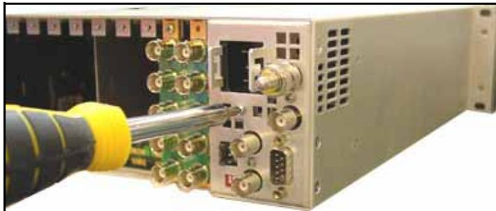
**Figure 5-1** Removing the Rear Panel PSU Screw
