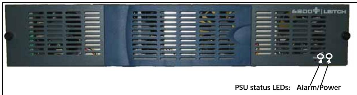
**Figure 5-3** Location of PSU Status LEDs
