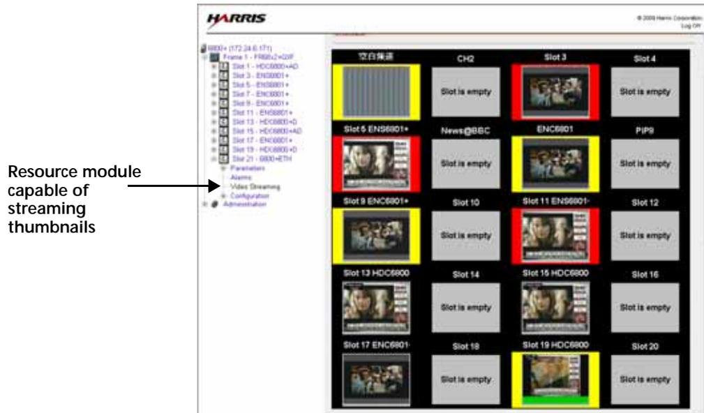
**Figure 4-22** 6800+ETH Streaming in the HTTP Control Interface
