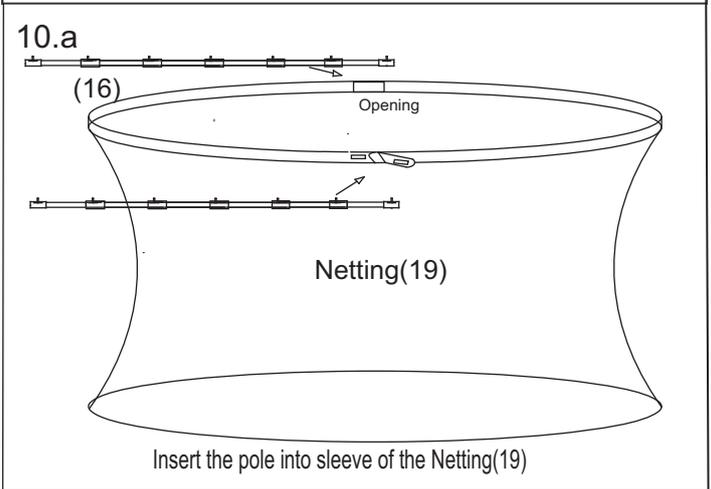
11. Joint each end of Top G4 Pole (16) by the clip of connector at each opening. The Top Sleeve of the Netting (19) become a round shape.
