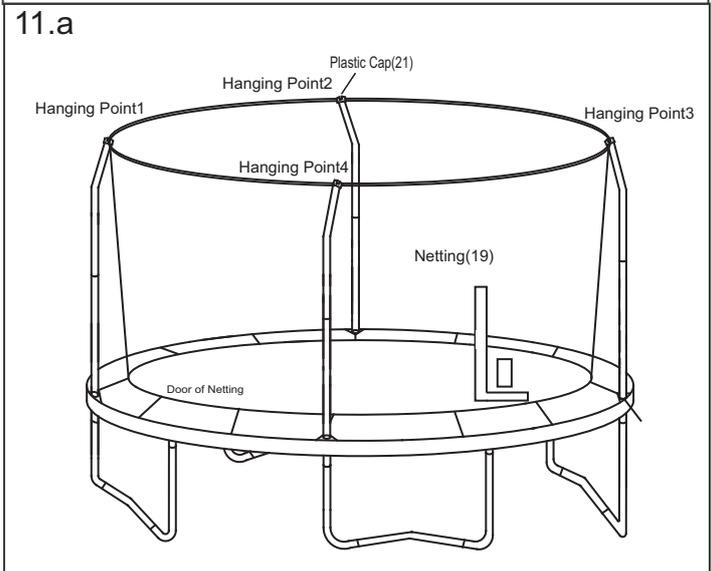
12. Note: During steps 11 and 12, you will “sew” the lower edge of the Netting(19) to the V-rings on the bed using the Cords(22).
