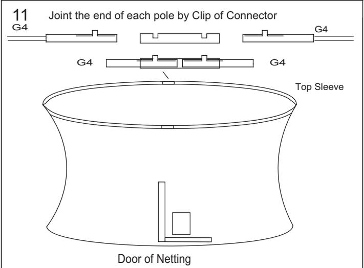
See insert drawing for attached of G4 Pole (16):
