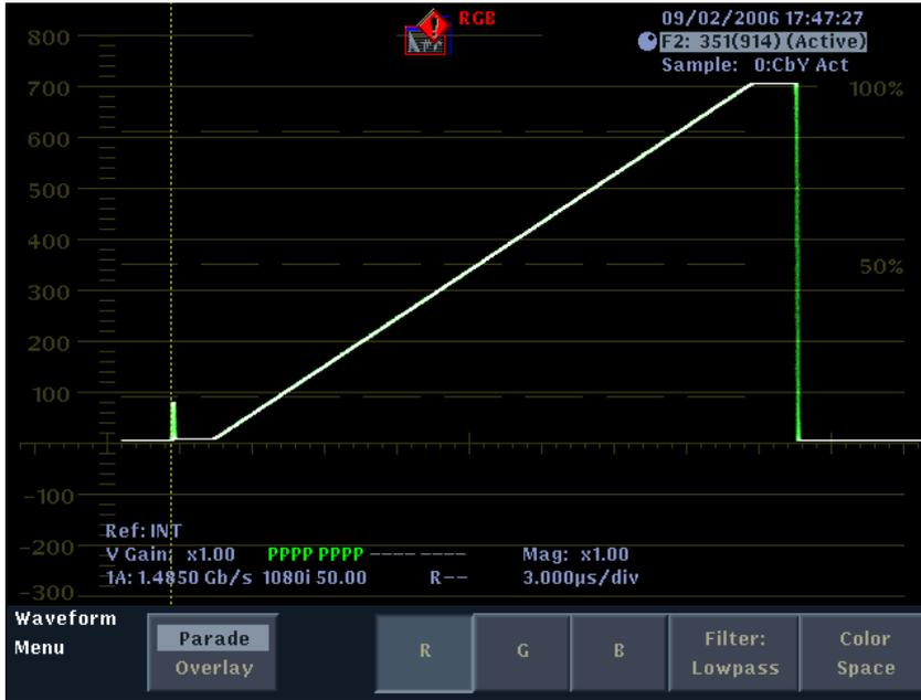
Figure 4-5 - Hard Clipped Output
