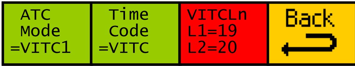
To set up timecode extraction, select the timecode type from VITC, LTC or ATC and if necessary, select the ATC mode or VITC line numbers to further specify where the timecode data should be extracted from.
