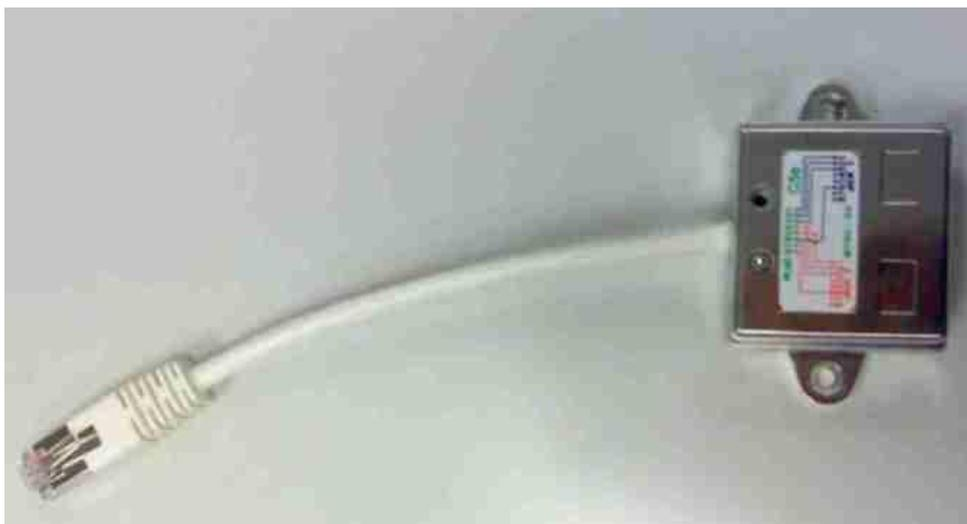
**Figure 10-2 GPI Splitter. Has 2 RJ-45 Sockets, one for the Comms and one for the GPI's**
