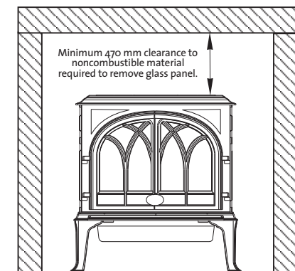
Figure 6. Clearance for glass panel removal.
