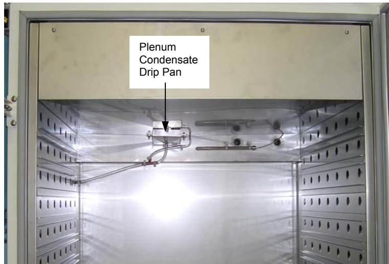
PLENUM COVER INSTALLED
