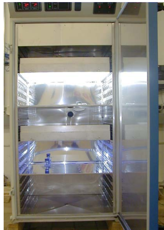
CEO932 Photostability Test Chamber - Cover Panels Removed
