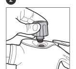
Remove Pressure Locking Safety Cap. The Continuous Steam Lock should be in the "Unlocked" position.
