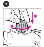
Push down on the Pressure Locking Safety Cap until the cap "clicks". While cap is pressed, turn counterclockwise to remove.
