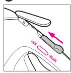
To access continuous steam push the Continuous Steam Lock to the "locked" position.
