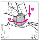
WAIT AT LEAST 3 MINUTES BEFORE REMOVING THE PRESSURE LOCKING SAFETY CAP. This allows the pressure inside the tank to dissipate.
