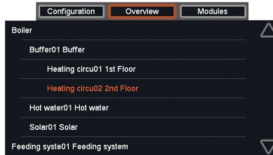
Represents all components of the system with their designations in hierarchical order. Subordinate components are thus set back (e.g. the "1st Floor" heating circuit is attached to the buffer). The component designation can be edited by pressing on the list entry itself. The service technician can also edit the hydraulic assignment (to the boiler or buffer) on this page.
