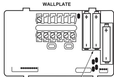
INSTALL 3 AA ALKALINE BATTERIES
