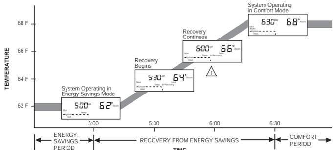
THE THERMOSTAT USES THE SAME SCHEME TO RETURN TO LOWER COMFORT TEMPERATURE DURING THE COOLING SEASON.
