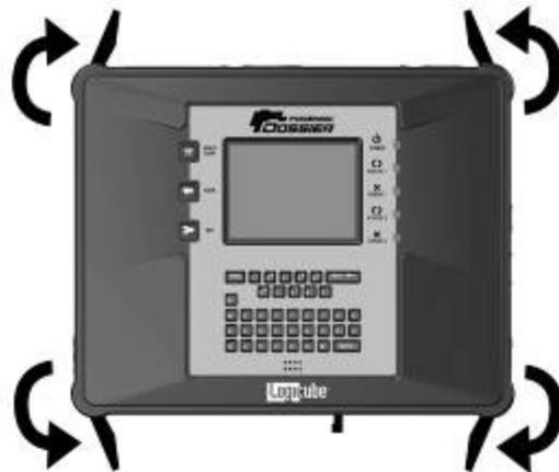
**Figure 8, Opening corner latches.**
