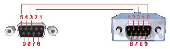
Only Pins 2 (RO), 3 (TX), and 5 (Ground) are used on the RS-232 serial interface.
