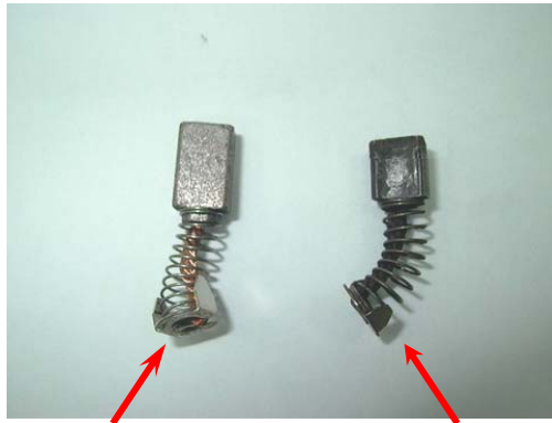
New Motor Brush Worn Motor Brush (Fig 41)
