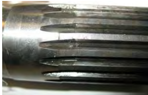
Figure 1: A slightly twisted shaft. The device must be able to verify that the shaft is twisted.
