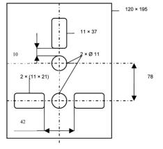
Mount the reel on a solid structure that is capable of withstanding load of max. 2,500 kg). To mount the
