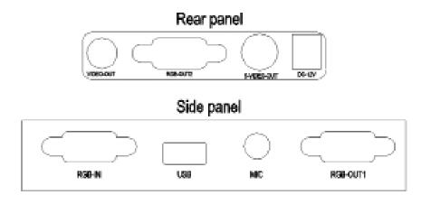
DC-12V IN: External 12V power adaptor input connection
