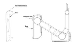
Install visualiser on the wall and position the camera head vertically to the base. (Need to take close-up lens off first)
