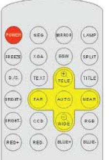
**SPLIT**: Press the "SPLIT" button and the image will be split into two images. One is the live image and the other is a frozen image. Press the "SPLIT" button again to exit
