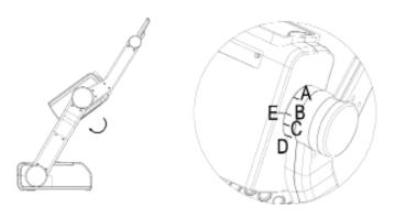
**ATTENTION**: When mark E is in line with A, the camera head and the base are parallel. When mark E is in line with mark D, the camera head and the base are vertical. When the visualiser is folded, mark E is in line with mark C
