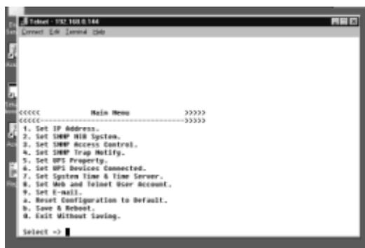
Fig.40. NetAgent Telnet window
