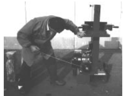
Fig.9 Petrol or diesel engine start-up
