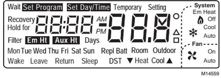
Fig. 12. LCD segments display.
