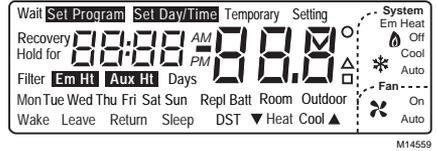
**Fig. 10. Display of all LCD segments.**
