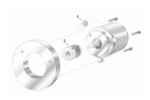
Install the encoder with fixing clamps (ordering code LKM 386):
