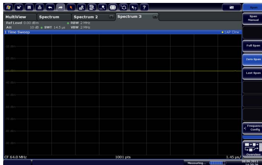
Fig. 3-10: Time domain display of the calibration signal
