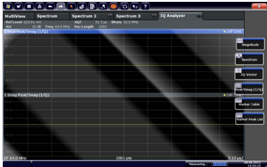
Fig. 3-11: Inserting a Real/Imag diagram for I/Q analysis
