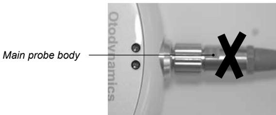
This will result in damage to the probe and will invalidate the probe warranty.
