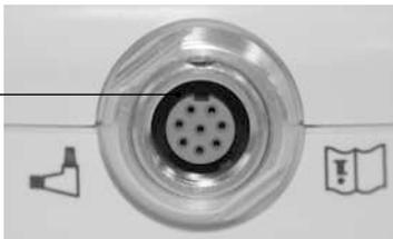
2.8.c The arrow at the front of the probe plug indicates the position of the 'key' and should be aligned with the front of the Otoport.
