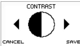
2.7.9.a Pressing the **Contrast/Delete** key while the logo screen is shown following switch on allows the user to adjust the screen contrast.
