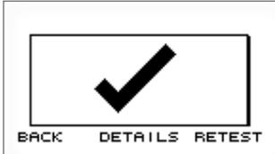
12.2.1.c The levels recorded at all frequencies are within the absolute range and within  $\pm 3\text{dB}$  of the probe specific values.
