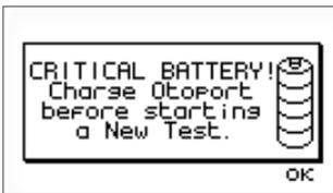
16.4.2.a When the battery power reaches 5% remaining a **Critical Battery** warning message will appear on screen. This equates to approximately 10 minutes of use. Select **OK** to accept the message and return to the previous screen. It will not be possible to start a new test when the Otoport has reached this level of charge. The Otoport should be charged as soon as convenient.
