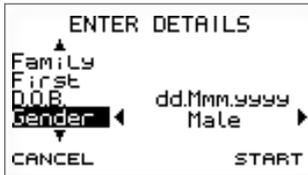
2.7.6.a Left and right arrow keys are used to move through choice bar options. For example when entering patient details in the **Gender** field, pressing the right arrow key will rotate the selected option between **Not Given**, **Male**, **Female** and **Unknown**. Choice bars options are enclosed by arrow graphics.
