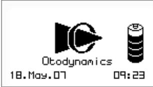
16.4.a When the Otoport is switched on, the opening screen shows a battery indicator which displays the remaining level of battery charge.
