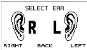
5.7.1.a The **Select Ear** screen represents the patient facing you. By defaulting to a **No Ear Choice** the **Select Ear** screen forces the user to choose an ear before the test can be saved. Press the right control key or the right arrow to select the **Left Ear** or press the left control key or the left arrow key to select the **Right Ear**. Select **Back** to return to the **Patient details** screen.
