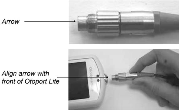
2.8.d It is possible to feel when the probe key is aligned as the probe will mate with the socket easily. Push the probe into the socket until it hits the end stop. DO NOT force in the probe.
