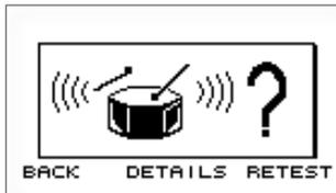
12.2.1.i There was significant noise during the calibration test. This noise may have influenced the levels recorded so a **Retest** should be performed.
