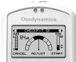
2 A vertical stimulus needle and low noise, with two blue LEDs, indicate a good probe fit. Press to **START** the test.
