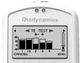
3 An OAE histogram is continuously updated during the test. The symbol indicates that a band meets pass criteria.
