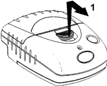
10.7.c Unwind a small amount of paper from the roll. Insert the new roll (2) ensuring the paper will pass through the paper feed (3) and close the cover with a click.
