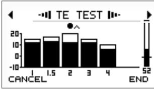
5.5.1.o Select **Cancel** at any time during a test to pause the test. This may be useful if the ambient noise increases. **Cancel Test?** is displayed at the top of the screen and three options are provided. **Yes** will terminate the test; **No** will continue the OAE recording and **Checkfit** will restart the test at the Checkfit stage.
