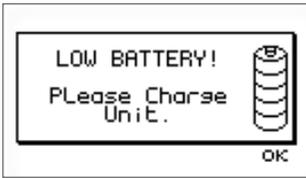
16.4.1.a When the battery power reaches less than 10% remaining a **Low Battery** warning message will be displayed. This equates to approximately 30 minutes of testing time. Select **OK** to accept the message and return to the previous screen. This screen will continue to appear every minute, as a reminder to charge the battery.
