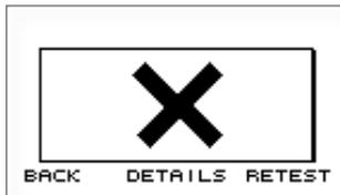
12.2.1.e One or more of the levels recorded are outside the absolute range specified for the probe. If a Fail is shown on screen inspect the probe coupler tubes for debris, replace the coupler if necessary and repeat the Probe Test, by selecting **Retest**, ensuring the ear piece is firmly inserted in the test cavity. If the test continues to fail there may be a fault with the probe or system. Contact your dealer or Otodynamics for advice.
