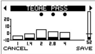
5.7.a When a test is completed, select **Save** to save the result. Select **Cancel** to discard the result; a confirmation screen is provided which also gives the option to restart the test at Checkfit.
