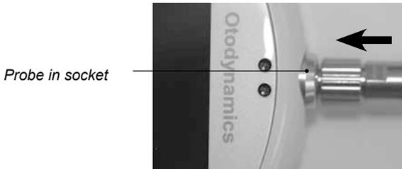
2.8.e Screw up the **knurled sleeve** in a clockwise direction until finger tight.
