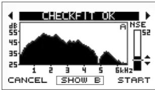
5.4.3.a Press the left and right arrow keys during **Checkfit** to access the **Stimulus Spectrum Display**. This shows how the energy in the stimulus waveform is distributed over frequencies. This distribution is dependent on the fit of the probe and the geometry of the individual ear canal.
