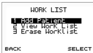
6.3.a The **Work List** facility allows for **Patient Details** to be entered and saved prior to the test, to reduce data entry time during the testing session.
