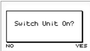
3.1.B Select **Yes** to confirm Otoport switch on, or **No** to turn the unit off again. If **Yes** or **No** are not selected within two seconds of pressing the on/off power key, the device will automatically turn off. The unit will turn off if any key other than **Yes** is selected. This is to prevent accidental switch on during transit.
