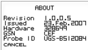
7.5.a The **About** screen details information relating to the Otoport's identification and mode of operation. The firmware revision number and creation date is stated together with the unit's unique hardware ID. If a probe is connected the **Probe ID** will also be displayed for reference.
