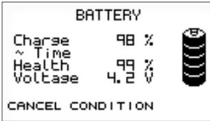
7.3.a The **Battery** screen provides information on the current battery status. The total **Battery Power** remaining is displayed as a percentage and as an approximate operation time. The calculated time is only an approximate indication as the power requirements will vary depending on the mode of operation.
