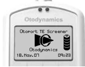
3 Date, time and battery status are displayed while system checks are performed.
