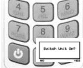
2 Press the button to turn on the Otoport. Confirm within 2 seconds by pressing the button.
