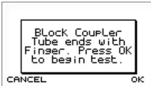
12.3.2.a If the probe coupler is not fitted correctly, sound may leak between the probe loudspeaker and microphone. The **Occlusion Test** helps to check that the probe is assembled and is performing correctly.
