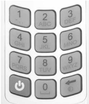
2.7.3.a Character entry is similar to a mobile phone where numbered keys can be pressed sequentially to select the required character.
