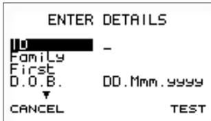
5.3.a The **Enter Details** screen allows patient data to be entered and saved with the test record.
