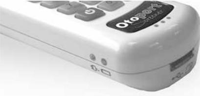
16.5.2.b **Power light** - The green light below the plug symbol shows that the device is powered.
