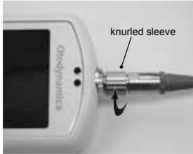
1 With the arrow at the front, connect the probe and screw the knurled sleeve until finger tight.
