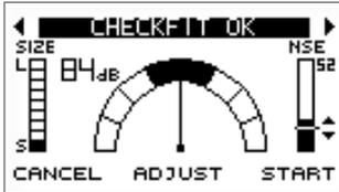
5.4.1.a It is important to perform a test in the appropriate conditions. The **Checkfit** screen allows a user to assess the testing environment before starting the test.
