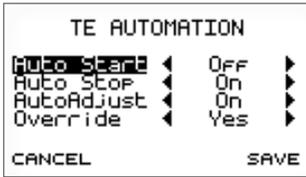
9.2.3.a The Otoport Screener has programmable automation logic to enable the user to configure the test routine to their preference. The test process can be set to be fully automated or manually operated, depending on the desired control over the test.
