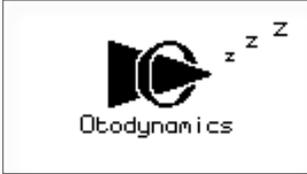
16.3.a To save power, the Otoport will go into standby mode after 3 minutes of inactivity. The standby screen will be displayed.
