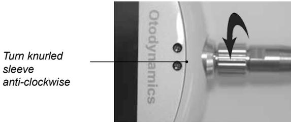
2.9.b Then gently pull the probe out of the probe socket.
