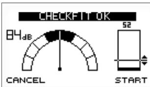
9.2.3.e With **Auto Start Off**, it is necessary for the user to select **Start** to begin recording from the **Checkfit** stage.
