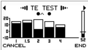
5.5.1.a Test data is displayed graphically on the histogram screen in ½ octave bands: 1k, 1.5k, 2k, 3k and 4 kHz. The clear section of each band represents the OAE signal level within each band and the shaded section represents the noise level at that frequency.
