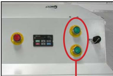
The **Vacuum Pump Switches**, highlighted above come standard if the Vacuum Table is purchased with the machine.
