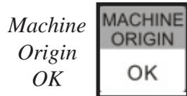
This will cause the machine to first move the Z-axis to the top of travel. Then the X and Y axis will move simultaneously, to the home / reference position. A sensor on the gantry is used to locate this position.
