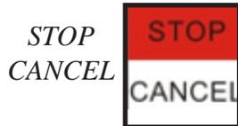
This will abort the sequence and the machine will stay still. There will be no reference position and break points, offsets and all functions that rely on a reference position will be invalid.
