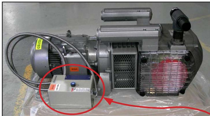
If a Vacuum Pump/Blower was part of your order, you will have an electrical starter box that looks like this. You should not need to wire the Vacuum Pump/Blower Motor, it has been wired and tested at the factory.
