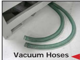
Use the T-Connector to connect the Blue Hose to the 2 Vacuum Hoses to the Machine.
