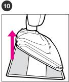
When unit has cooled, remove Ultra-Microfiber Pad and water tank. Store unit upright in a dry area.
