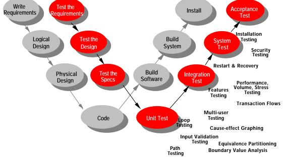
Figure 5 – Dynamic test in the lifecycle
