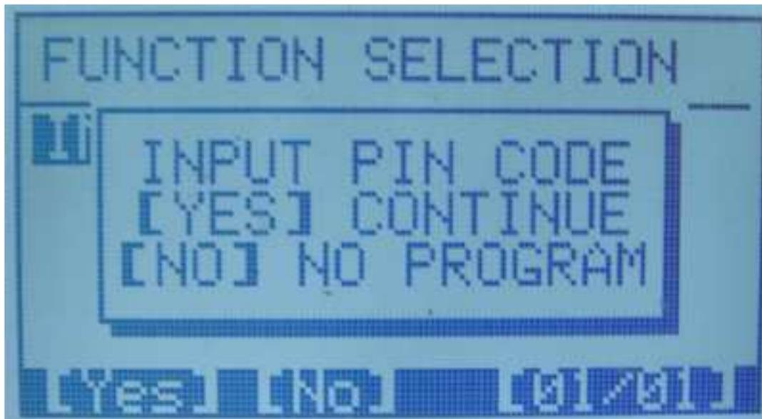
Press [YES] input PINCODE, press [NO],no the program functions.
