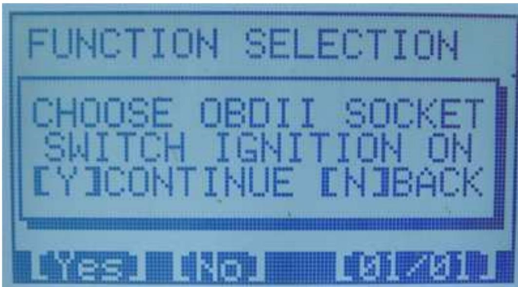
Choose OBDII socket, and switch ignition on, Press [YES] continue->
