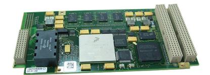
The EM9A is a complete embedded SBC for use on any carrier board in different industrial environments. The final application consists of a stand-alone EM9A or an EM9A with an application-specific carrier card.
