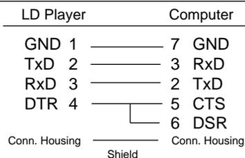
The CC-03 is an RS-232 cable which interfaces Pioneer's LD-V8000, LD-V4200 and LD-V2200 videodisc players and the LC-V330 AutoChanger to the IBM InfoWindow\*, the Apple II series Super Serial Card and to Pioneer's UC-V102 Videodisc Controller.
