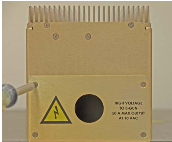
Figure 2-7 Removing the FPS Conduit Panel
