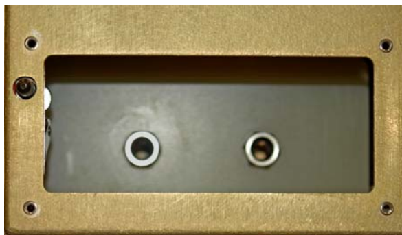
Figure 2-9 FPS Receptacles for Banana Plugs on HV Output Cables
