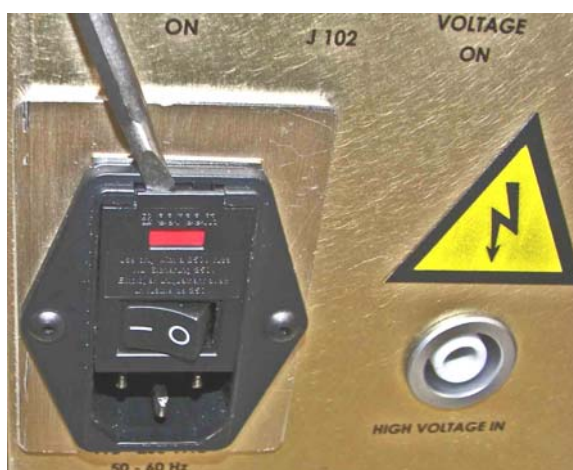
Figure 5-5 Prying Open the Fuse Block's Cover
