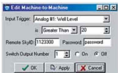
Figure 5: Turn Pump Off is Level is Greater than 20 feet
