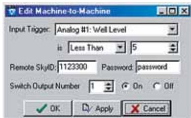
Figure 4: Turn Pump On if Level is Less than 5 feet
