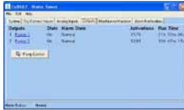
Figure 2: Output properties showing pump control
