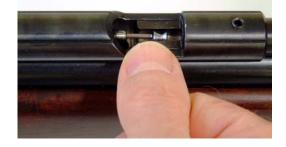
2. Insert a **pellet** of the proper caliber into the open breech. Make certain the pellet enters *nose-first with the fan-tail skirt to the rear*, as shown.
