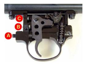
The QB78 trigger features three adjustments:
