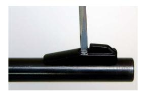
7. If desired, use a *1/8" flat-bladed* screwdriver to remove the front sight.
