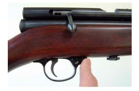
8. Release the **Safety**, by rotating forward and out of the trigger guard.
