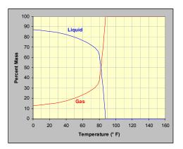
The *critical temperature* of CO<sub>2</sub> is **87.8°** F and this temperature is of particular importance to air-gunners. As shown in the graph above, below this temperature both gas *and liquid* CO<sub>2</sub> coexist in the Powerlet. Above this temperature, only *gas* can be present. The cartridge exhibits a natural pressure-regulating mechanism, but <u>only at temperatures lower than  $87.8^{\circ}$  F.</u>
