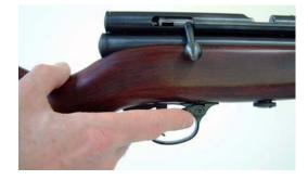
2. Apply the **Safety** by swinging it to the rear as shown above.
