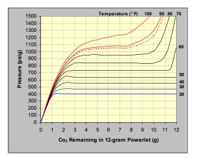
$CO_2$  regulation is summarized below. Mark the ambient temperature on the horizontal scale and read the corresponding pressure and mass limits directly above it. For example, on a 70° F day, a regulated pressure of 840 psig will be provided as long as the Powerlet holds at least 2.8 grams but not more than 10.6 grams of  $CO_2$ . Hence the first few shots will be "hot" until you use 1.4 grams from a new Powerlet. You will "run out of liquid" when 2.8 grams of gas remain in the cartridge.
