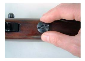
2. Unscrew the **Locating Screw Nut** and remove the action from the stock.
