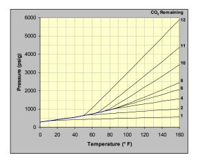
This figure presents the pressure within a Powerlet as a function of temperature with from 1 to 12 grams of  $CO_2$  remaining in the bottle. Note the blue segment partially common to all of these traces; this is the *saturation line*. A  $CO_2$ charge of 6.55 grams remaining in the 14 cc cartridge volume (0.468 g/cc) will exhibit a pressure-versus-temperature curve that follows the *saturation line* all the way to 87.8° F; all other charges depart from the blue line at a *lower* temperature.
