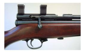
2. Mount the bases to the receiver. Only handtighten the clamp screws; you need the bases to slide freely at this point.
