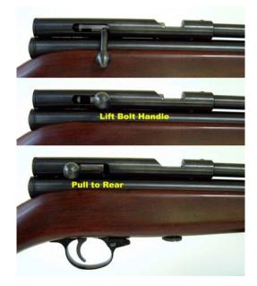
3. Open the **Bolt** as illustrated above. Opening the bolt leaves the loading chamber open to inspection. More importantly, *retracting the bolt prevents dangerous accidental piercing of the rearward-facing CO*<sub>2</sub> *cartridge*.
