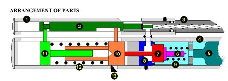
The **Breech Tube** (1) contains the **Bolt** (2) and is attached to the **Barrel** (3) by a setscrew and O-rings. It sits atop the **Gas Tube** (4) to which it is screwed. An O-ring seals a gas transfer path between the **Valve Body** (8) contained in the **Gas Tube** and the firing chamber sealed by an O-ring on the **Bolt**.
