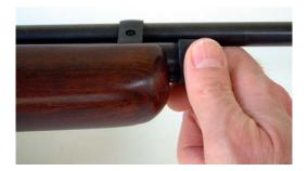
1. Verify that the **Gas Tube Cap** can be loosened *by hand*, as shown above. *Never* use a tool to rotate this cap. A tight cap indicates dangerously high gas pressure remains within the **Gas Tube**.
