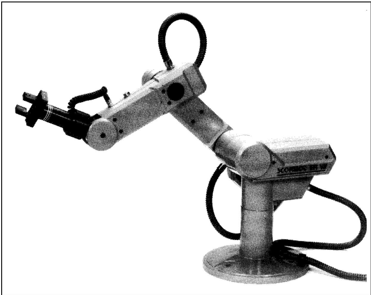
*Figure 2-1: SCORBOT-ER VII Robot Arm*
