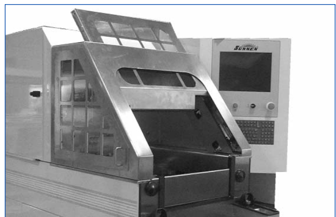
FIGURE-26, CE Work Area Cover
