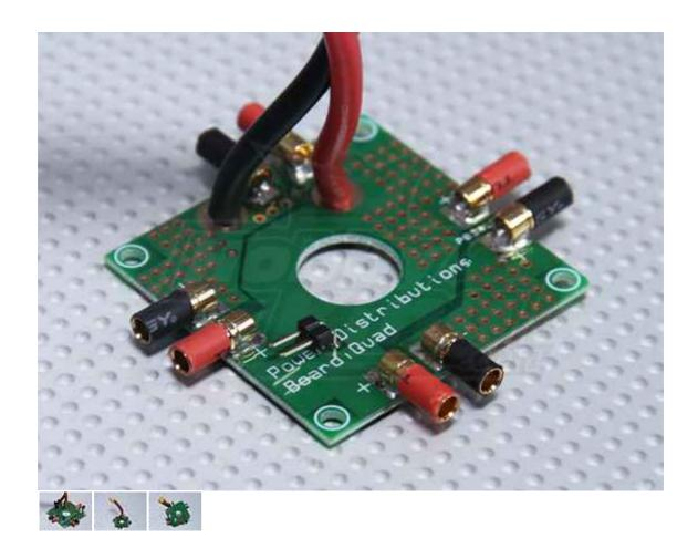
Designed in house by the HobbyKing Enginerds, this handy power distribution board has the same foot print as our Multri-rotor control boards and is the ultimate solution for tidy power distribution wiring. Simply use 3.5mm male connectors on your ESCs and plug a battery in. The PCB is Gold plated for optimality efficiency and also features a bling port (aka 2 pin JST size auxiliary power out) Perfect for powering LEDs or any accessory fitted to your Quadcopter.
