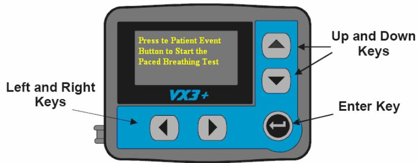
Figure 3.0 ANS Start the Paced Breathing Test
