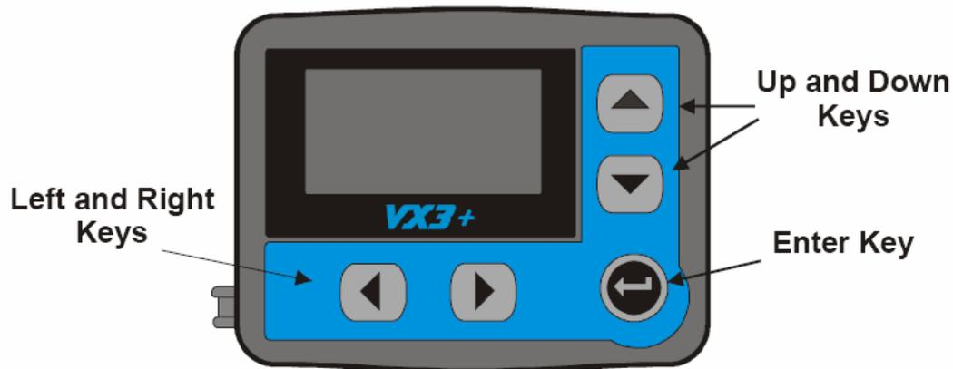
**Fig 1.1 VX3+ Holter recorder (Front)**
