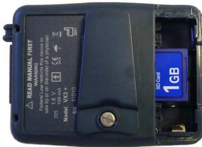
**Fig 2.1 Secure Digital Card Placement**
