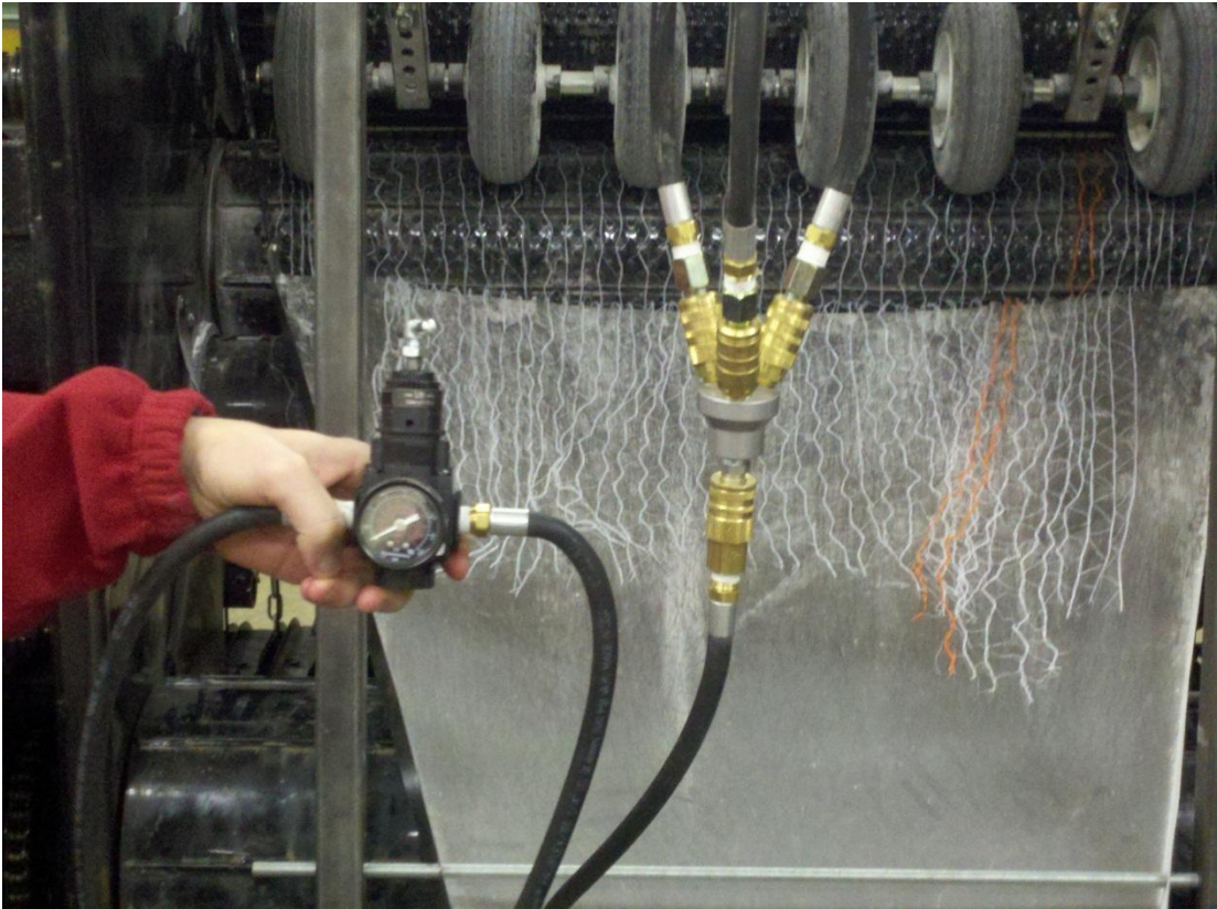
Figure 6: The pneumatic components of the design, leading to the air supply on left and 3 cylinders above
