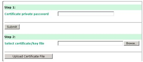
**NOTE** The WLAN certificate will remain after the AWK-3121 reboots. Even though it is expired, it can still be seen on the *Current Certificate*.
