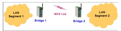
It is a good idea to plan your wireless network by drawing a diagram so that you know how each AWK-3121 is connected to other peer APs or wireless bridges by WDS, and how bridges are connected to other peer bridges by WDS. See the following figure for an example of a network-planning diagram.
