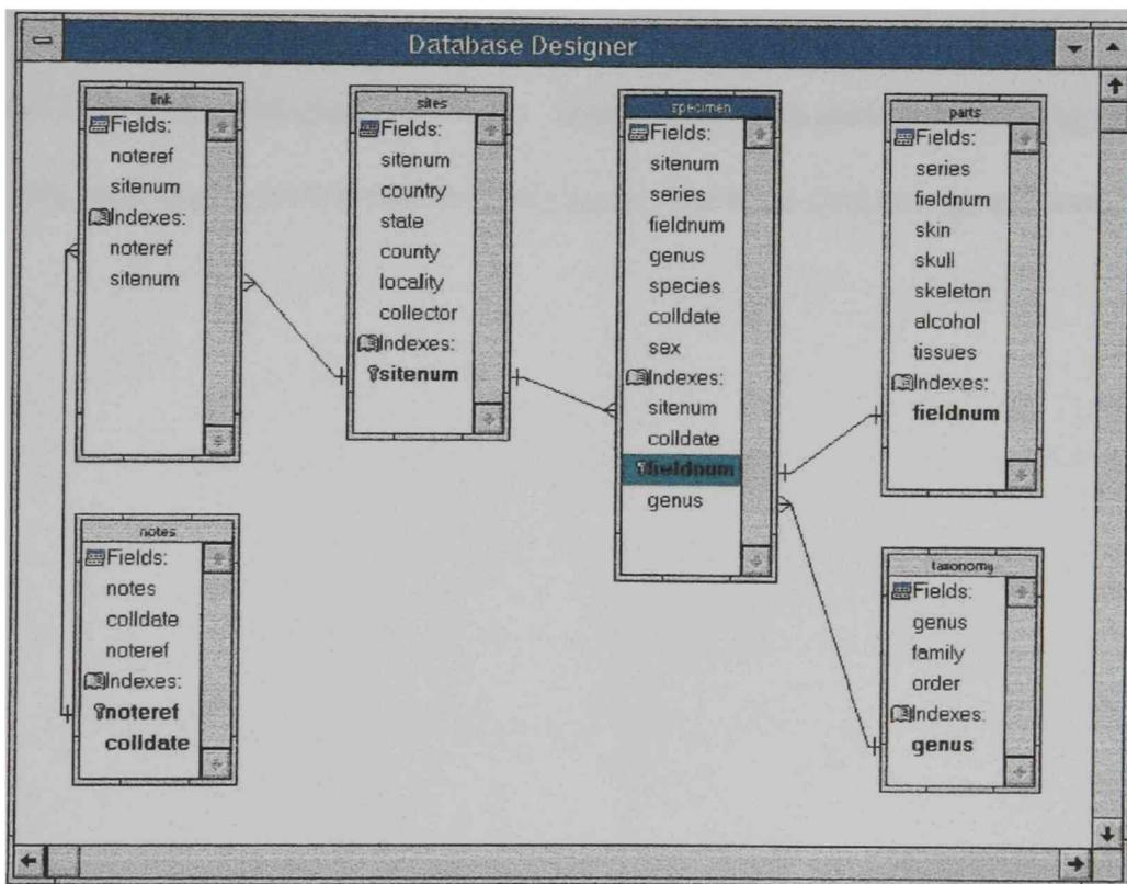
Figure 1. Relational database design schematic (partial) illustrating the linking of separate tables using key fields (in bold typeface).
