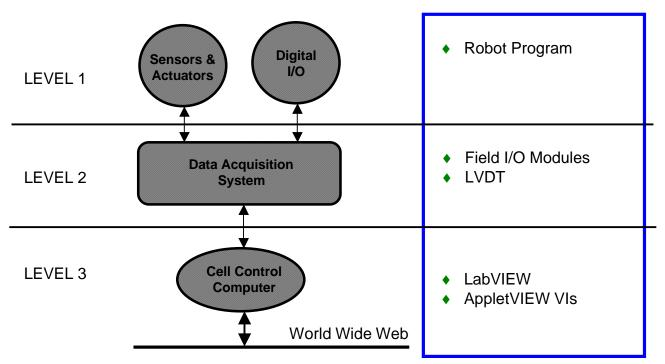
Figure 4. Software Framework for the Cell
