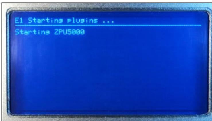
3. During Plug-in load up, the ZPU-5000 network address is displayed, in this case the E1 designation is used.
