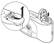
**4** Close the battery door securely. Slide it out to the side as far as it will go, press it against the camera base, and slide it back into the base to lock it closed. If you feel resistance, do not force the door. **Note:** Replace all four batteries when the low-battery indicator turns on, the LCD displays the low-battery message (**bL**), or the LCD status display does not turn on.
