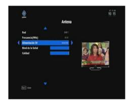
If you see a message like that in the screen, there is a short circuit in the aerial input. In this case, switch off the receiver and check the installation.
