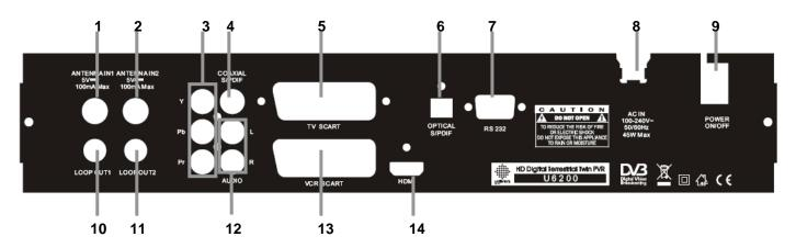
1 ANTENNA IN 1: Input for the first digital tuner
