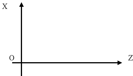
Fig. 1-2 X—Z plane rectangular coordinate system 2 (rear tool post coordinate system)
