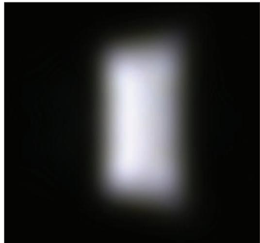
The beam pattern is rectangular (rectangle), good illumination uniformity, brightness difference is very little between the spot of the center and the periphery. There is almost no difference in the direction of extending the road completely with the continuous extension of the road, it is the ideal lighting lamp for road lighting.
