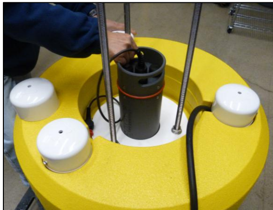
Figure 7-3: Replacing the RBP500
