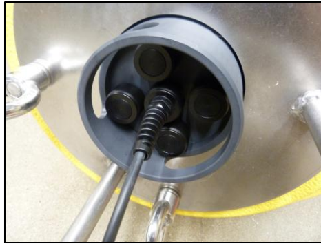
Figure 4-8: Sensor Connected to RBP500 Port P0
