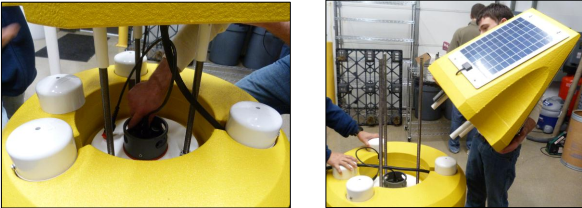
Figure 7-2: Disconnecting Power Cable from Port D and Removing the Tower
