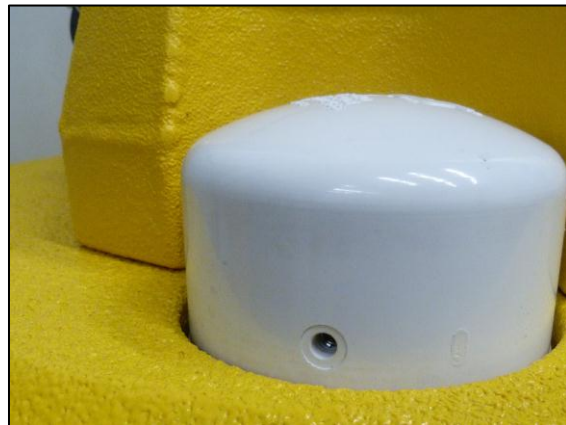
Figure 4-7: Pipe Cap on a Sensor Pass-through Tube
