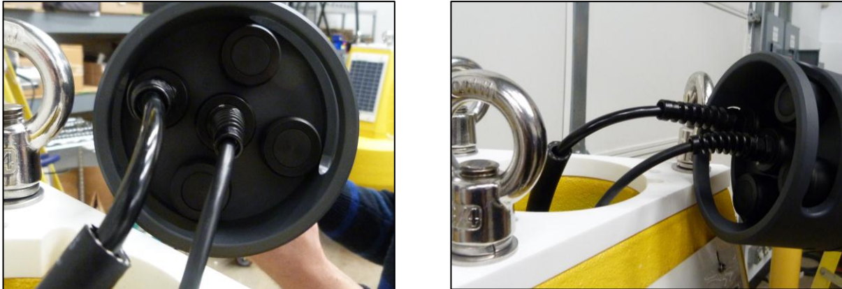
Figure 4-5: SDL500 Cable Connections and Installation
