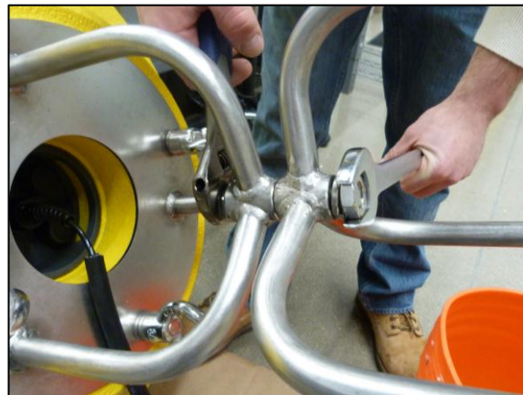
Figure 4-11: Securing the Cage Assembly
