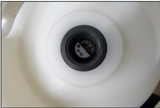
Figure 4-3: Top Port Pins and O-ring and Connecting SDL500 Antenna
