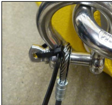
Figure 5-4: Cable Tie Installed on Bow Shackle
