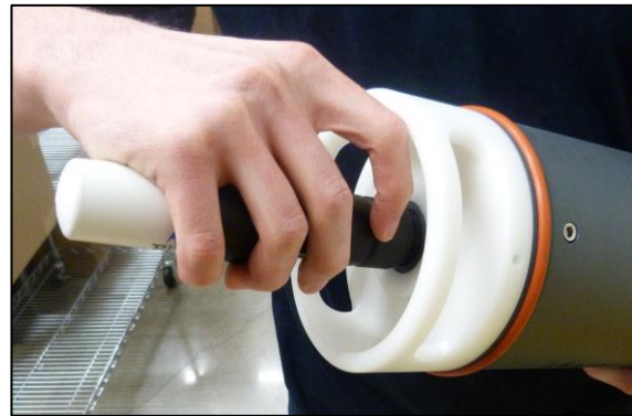
Figure 4-3: Top Port Pins and O-ring and Connecting SDL500 Antenna
