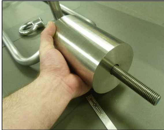
Figure 4-12: Inserting the Threaded Rod
