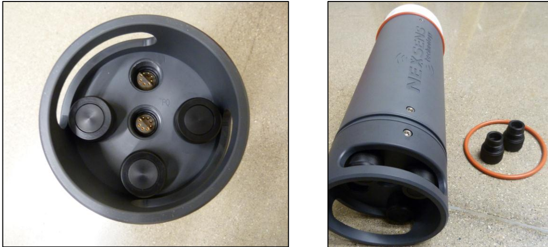
Figure 4-4: SDL500 with Port Plugs and Bottom O-ring Removed
