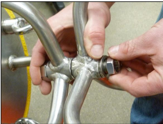
Figure 4-11: Securing the Cage Assembly
