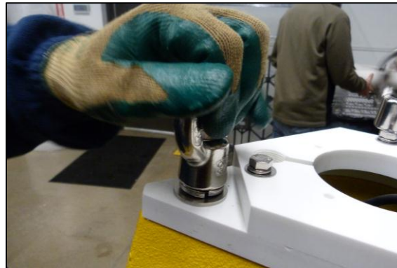
Figure 7-5: Tightening Eye Nuts
