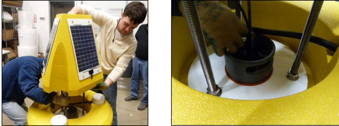
Figure 7-4: Reconnecting Power Cable to Port D
