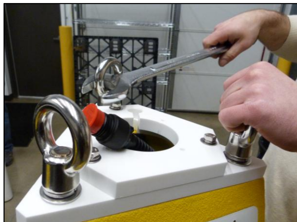
Figure 7-1: Loosen Topside Eye Nuts
