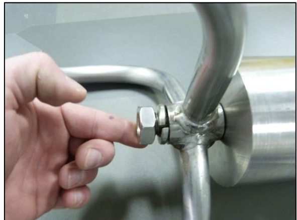
Figure 4-13: Securing the Ballast Weight
