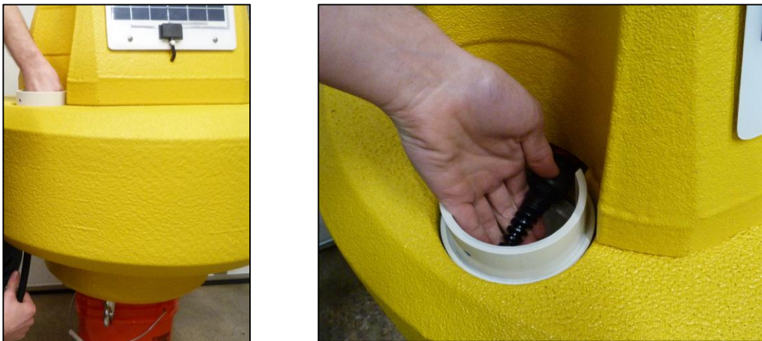
Figure 4-1: Feeding Sensor Cable into Buoy Tower
