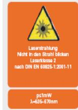
Laser class 2 warning labels on the laser instrument.
