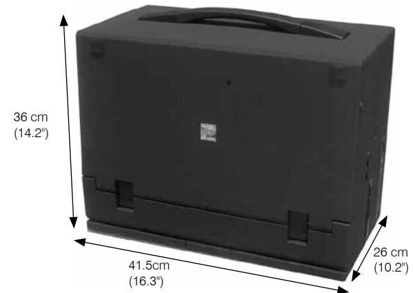
Figure 19-7: Dimensions of the box computer.
