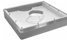
Figure 19-5: Tunnel for positioning the digital x-ray plate under the hoof.
