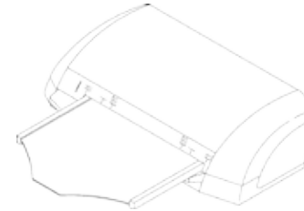
Figure 18-11: The notched end of the tray goes into the scanner. The smooth side should be up, providing a clear path from one end of the tray to the other.
