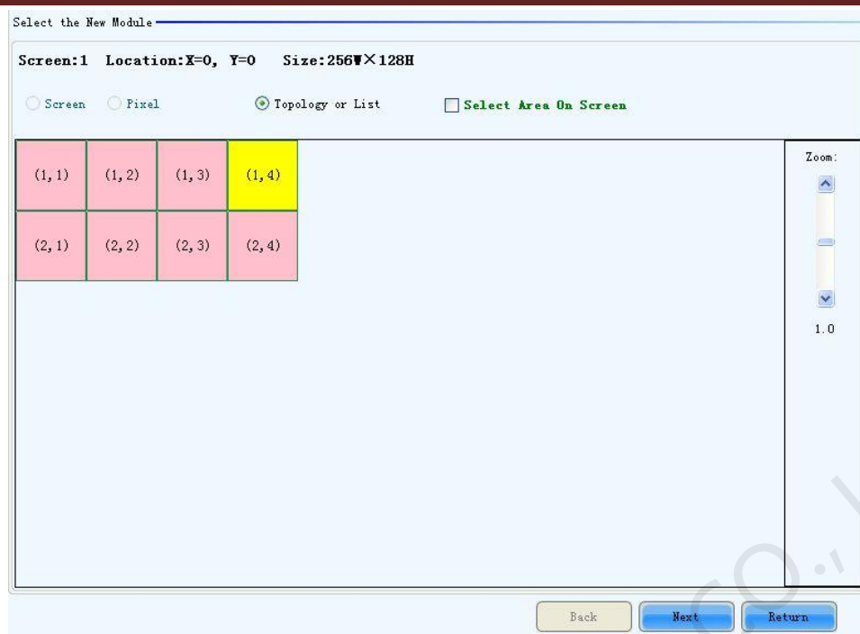
Fig. 5-89 the page for specifying the cabinet the new module is in
